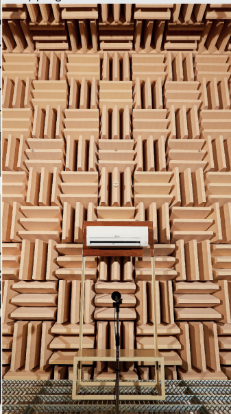
Anechoic Chamber Noise Test
